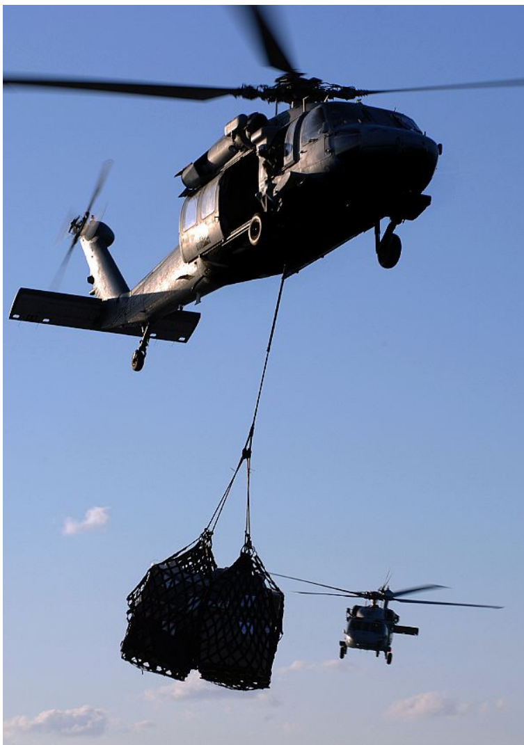
MEDITERRANEAN SEA (Nov. 18, 2007) An SH-60 Seahawk, attached to the "Sea Knights" of Helicopter Sea Combat Squadron (HSC) 22, transports cargo from the Military Sealift Command fast combat support ship USNS Arctic (T-AOE 8) to the Nimitz-class nuclear-powered aircraft carrier USS Harry S. Truman (CVN 75) during a vertical replenishment.
