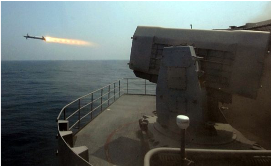
ATLANTIC OCEAN (Aug. 21, 2007) Nimitz-class aircraft carrier USS Harry S. Truman (CVN 75) conducts a test fire of the rolling airframe missile system (RAM). RAM uses missiles to shoot down incoming enemy aircraft.
